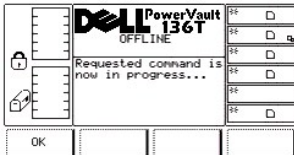
Figura 54. Diálogo Command > Drives > Unload > Command in Progress
