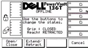
Figura 96. Diálogo Service > Library > Diags > Fingers > Step > Gripper Finger
