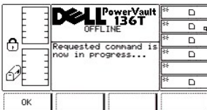
Figura 58. Diálogo Command > Drives > Reset > Command in Progress
